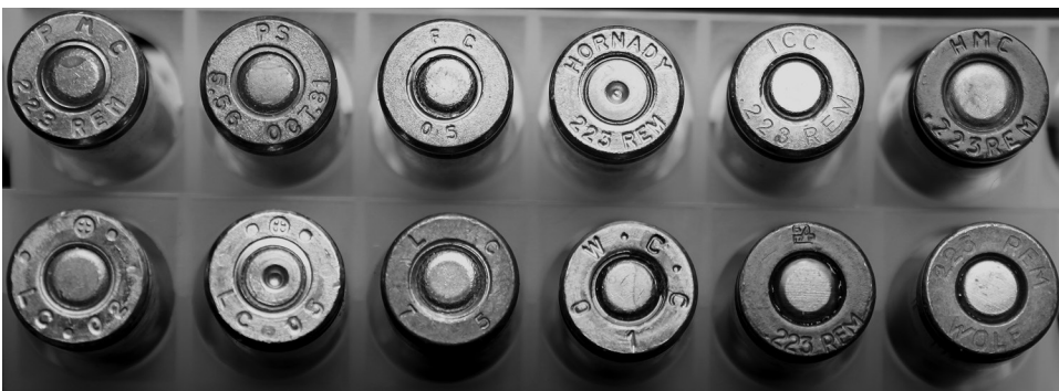
Figure 3.4 (See color insert.) An assortment of 5.56×45mm/.223 cartridge head stamps. Top row from left: Precision Metal Corp.; Poongsan Corp. Korea (October 1981); Federal Cartridge (2005); Hornady Manufacturing; International Cartridge Corp.; Hornady Manufacturing. Bottom row from left: Lake City Ordnance Plant (2002); Lake City Ordnance Plant (nickel plated) (2005); Lake City Ordnance Plant (1975); Winchester Cartridge Corp. (2001); Barnaul Cartridge Plant Russia; Wolf Performance Ammunition. (Image from author's collection.)
